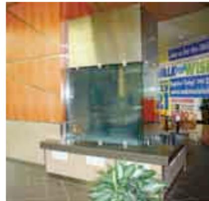
**FIRE SAFE** A 25-square-foot gas fireplace is completely enclosed by two layers of glass separated by a layer of air to keep curious tactile children out of harm's way.
