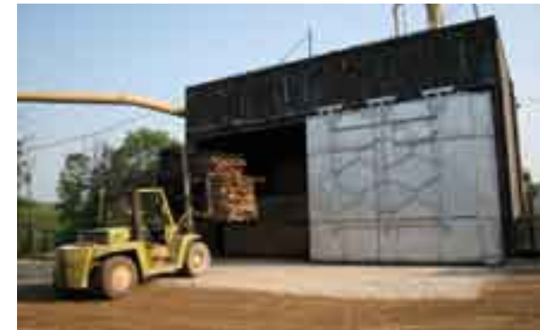
WOOD WORKS At Hardwood Lumber Company, a lift unloads a charge of timber in the kiln.
