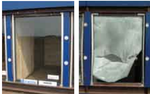
CATCHING A BREAK If a window with security window film breaks, the film holds the glass intact preventing shards from becoming lethal projectiles. The glass may shatter but will remain in or close to its frame.
