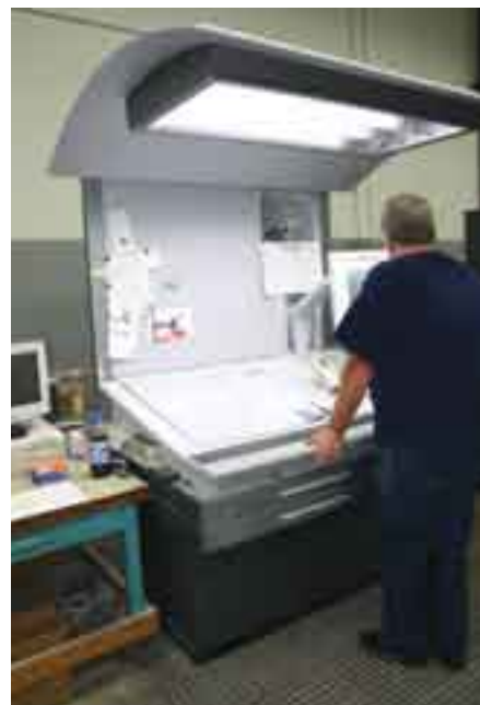
BRIGHT SIGHT Special fluorescent lighting allows for precise proofing of color prints in the press room.
