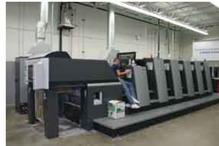
HEAVY DUTY Each of the company's Heidelberg printing presses weighs between 25 and 30 tons and, to work correctly, must not move at all. As the building site was unstable, much work was put into securing the foundation.
