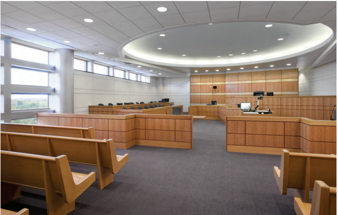
CLASSIC MATERIALS, CONTEMPORARY LOOK The walls behind the judge's bench are made of quartered cherry wood, as is the bench itself. The walls in the courtroom consist of large rectangular blocks outlined by linear grooves, called reveals.
