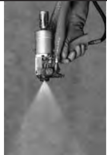
West Roofing applies Dow spray polyurethane foam (SPF) systems
