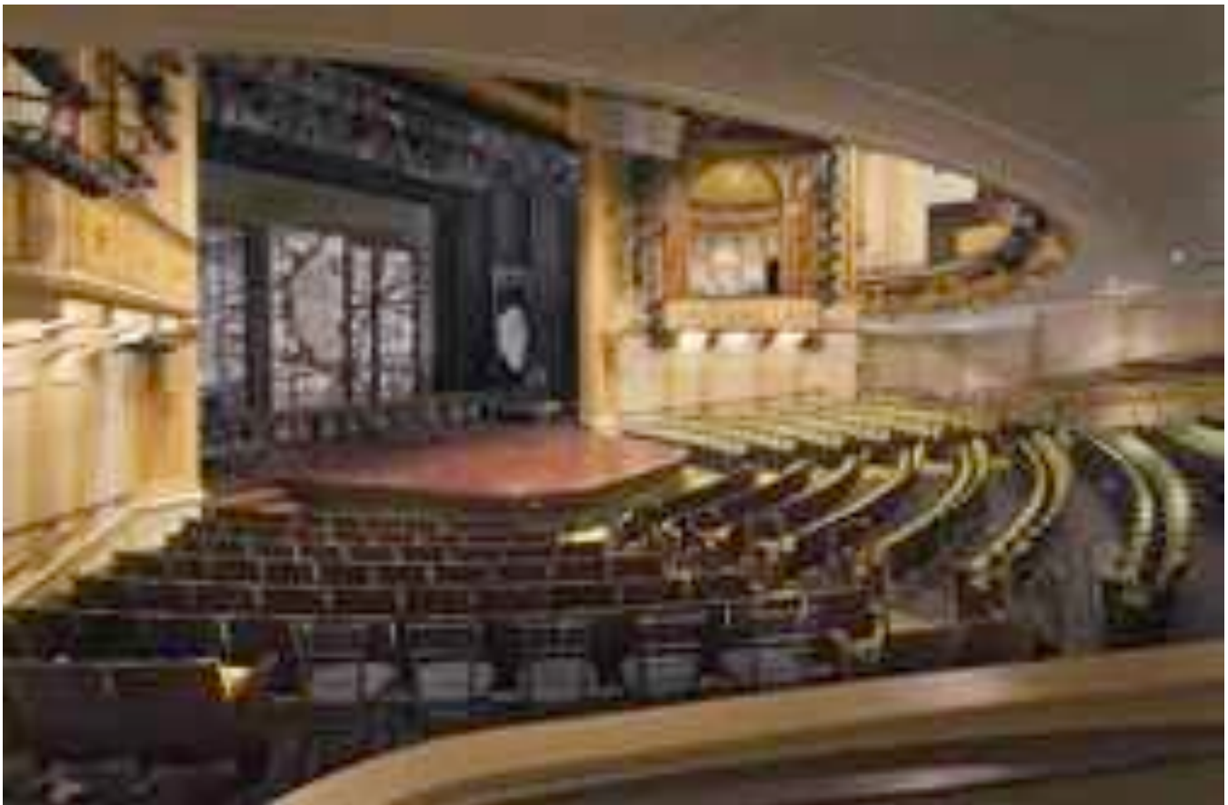
CENTER STAGE The focal point and most unique feature of the new Hanna is the thrust stage. Jutting out into the audience from the original proscenium stage, it promotes interaction between actor and theater patron.
